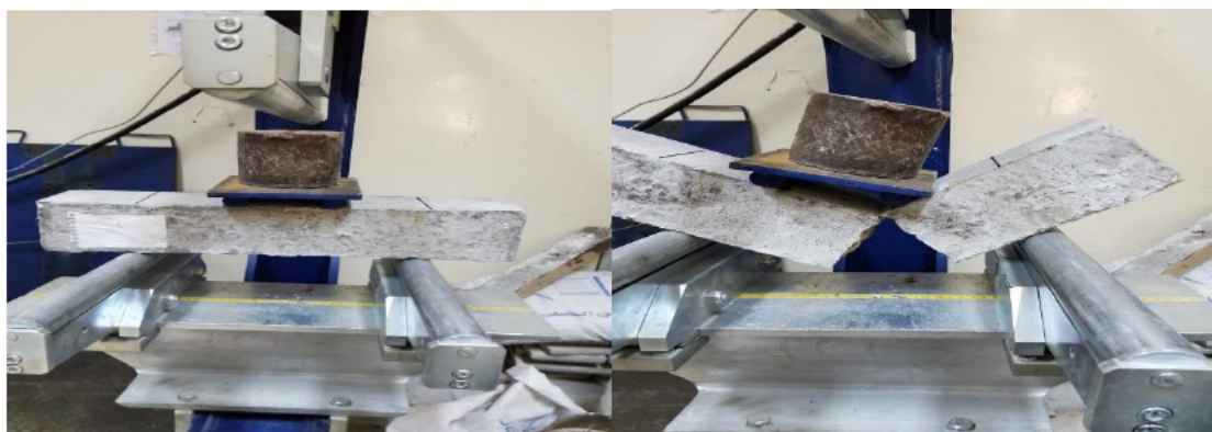
Figure 2-a Flexural Stress Test at Two Points.
