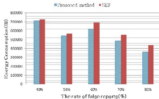
Figure 13 Energy consumption versus the rate of false reports (Fraction of compromised nodes = 3)
