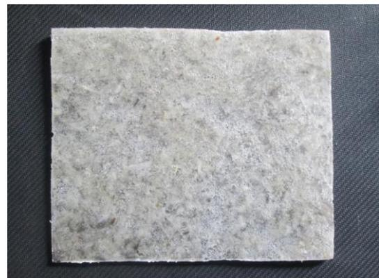
Fig 3: Epoxy Resin based Fish Scale Reinforced Composites after fabrication
