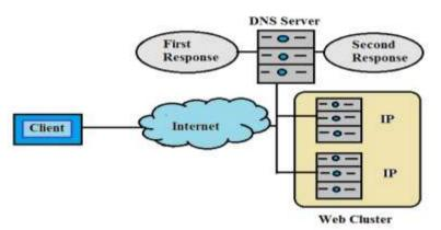
Fig2. Basic DNS Response for Redundancy
