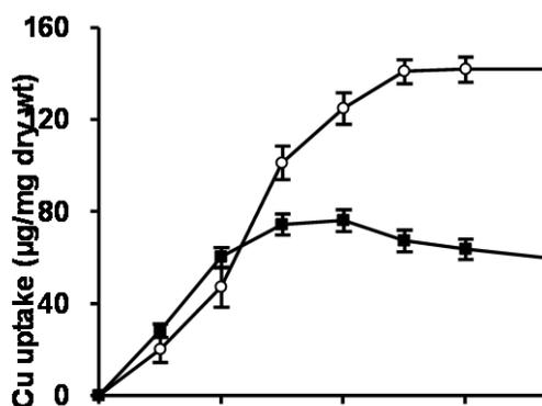
**Fig. 3:** Uptake of Cu per unit biomass of *Scenedesmus obliquus* (○) and *Synechocystis* sp. PCC 6803 at different metal concentrations.
