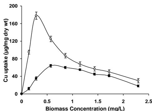
**Fig. 2:**Accumulation of Cu by *Scenedesmus obliquus* (○) and *Synechocystis* sp. PCC 6803 (■) at different biomass concentrations.
