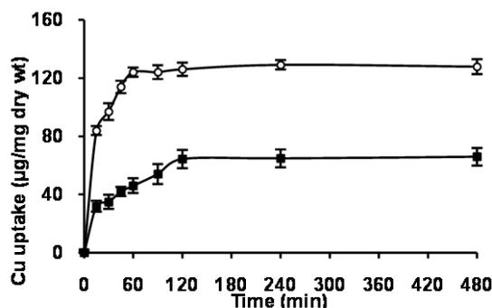
**Fig. 1:** Time-course accumulation of Cu by *S. obliquus* (○) and *Synechocystis* sp. PCC 6803 (■).
