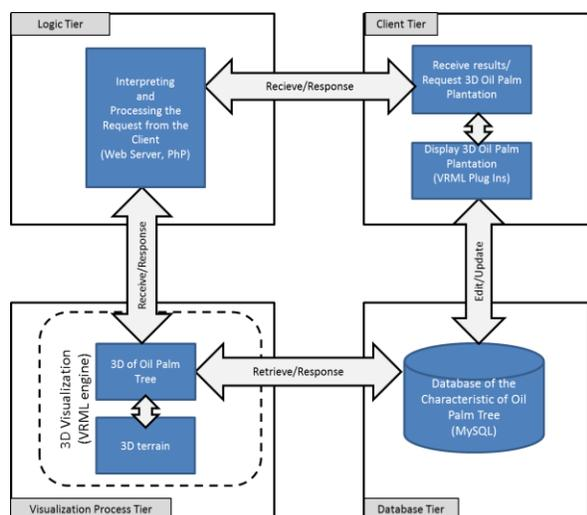
Figure 1 The architecture of a new four-tier framework
