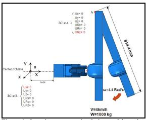
Figure 1. Low impact test simulation and boundary condition
