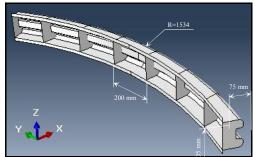
Figure 3. The strengthen ribs of bumper beam
