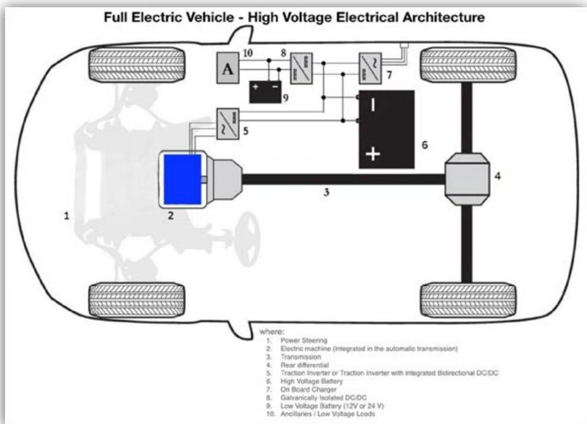
Fig. 3.1. Example of EV high voltage architecture representation.
