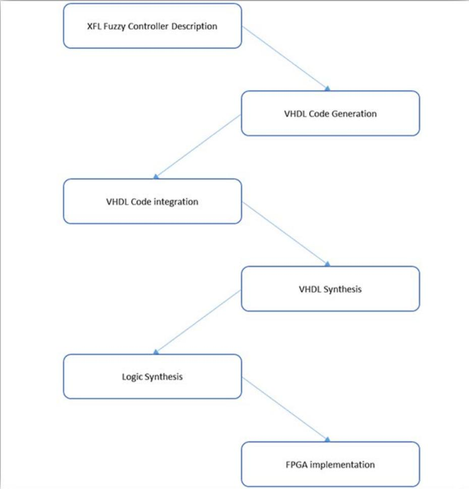
Fig. 4.1. Proposed design flow.
