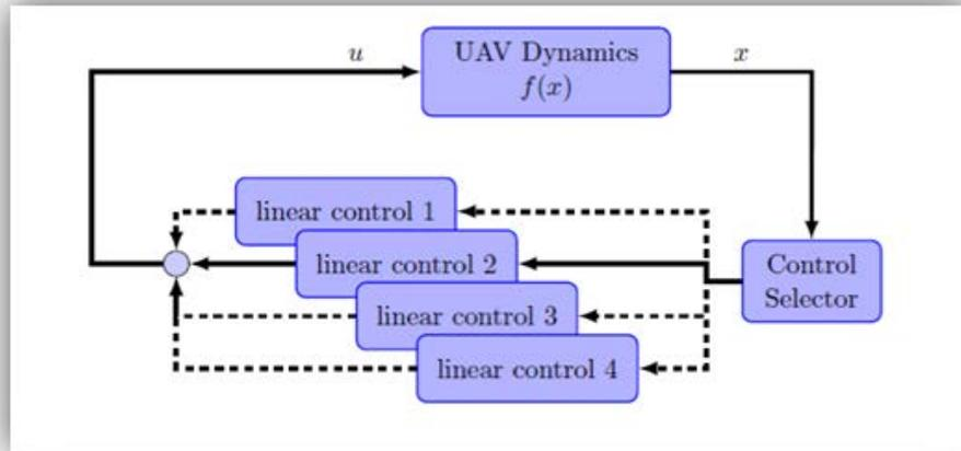
Fig. 2.3. Schematic of a gain scheduled scheme for UAV control [3].
