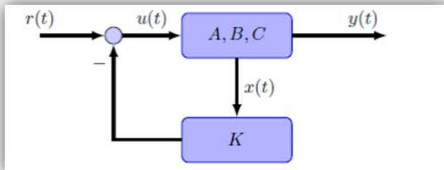
Fig. 2.2. Full-state feedback controller [2].
