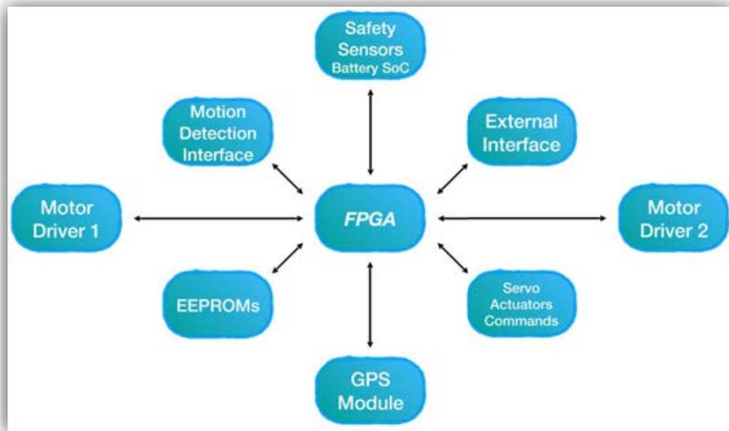
Fig. 5.2. FPGA's peripherals block diagram.
