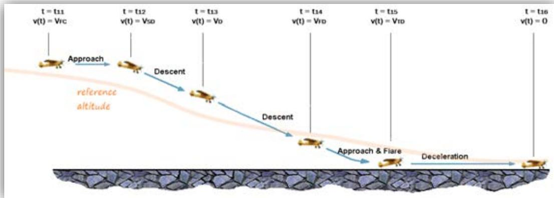
Fig. A.2. Reference landing manoeuvre altitude against vehicle's manoeuvre position, graphical animation.
