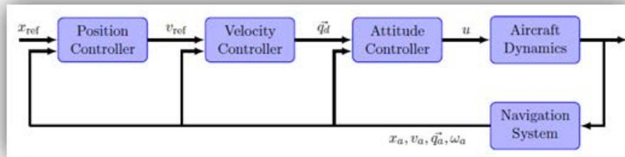
Fig. 2.1. Successive loop-closure control architecture [2].
