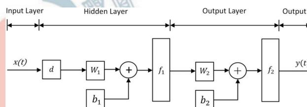
Figure 2. The FTDNN layout.
