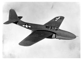
The first GE jet engine powered Bell's experimental XP-59 aircraft.
