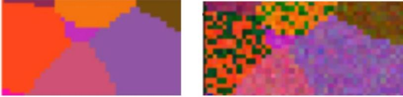
**Figure 15.** This figure shows the Euler angles in multiple grains of an example EBSD map as an RGB image. The image on the left shows the ground truth orientations. The image on the right shows the noisy map with up to  $15^\circ$  error in the Euler angles. The green pixels show the jumps due to the angle discontinuity at  $0^\circ$ - $360^\circ$ .
