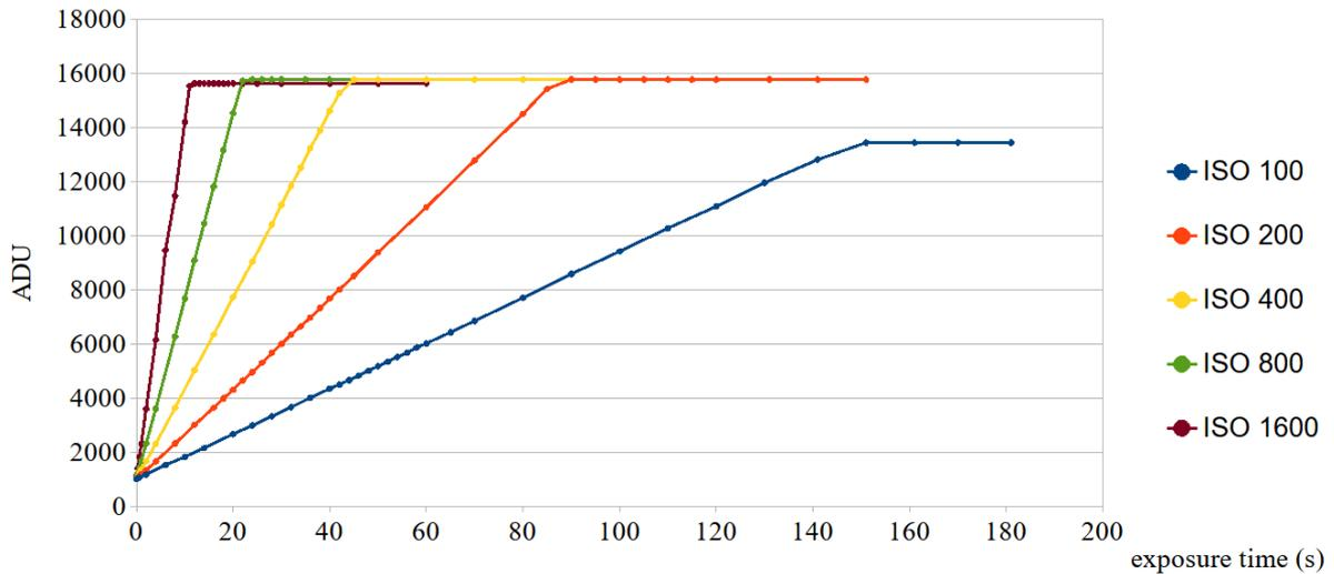
Figure 2: Canon 500D linearity at different ISO levels.
