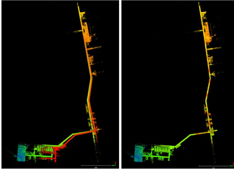
**Figure 4.** (Left) Output from ExplorerSLAM front-end. The robot started from the lower left corner and came back to the starting point. Color of the map indicates acquisition time. There is a significant misalignment between the starting and end part of the map (red and green). (Right) Output after Loop Closing back-end. The misalignment is corrected.
