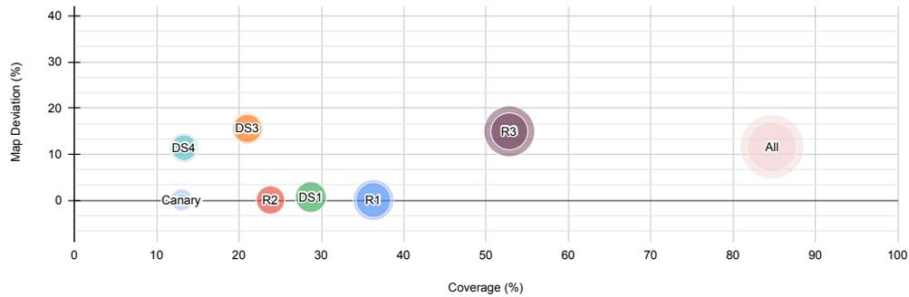
**Figure 28.** Impact Analysis per robot. The figure shows how much of the ground truth pointcloud was covered by each robot, and the mapping deviation accrued, both as defined by DARPA guidelines. The inner bubbles indicate how many artifacts were scored and the outer bubbles indicate how many were visited.
