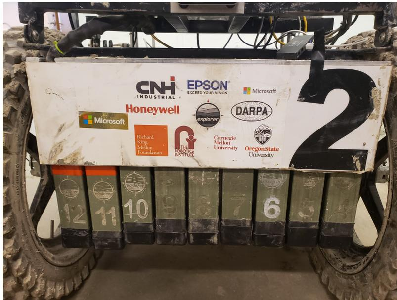
**Figure 20.** The communication node dropper onboard the R2 ground robot with 9 fiberglass node casings.
