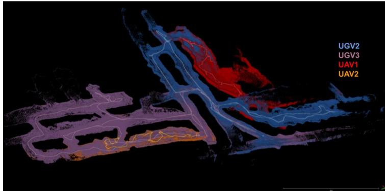
**Figure 6.** pointcloud maps produced by autonomous marsupial deployment of 2 pairs of ground and aerial robots. The colors correspond to the robot that captured the points.
