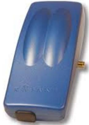
**Figure 19.** A Rajant DX2-50 radio (Rajant, 2023) that we used for communication between robots.
