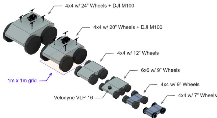
**Figure 2.** Graphic showing some of the different sizes considered for our ground vehicle platform. The larger sizes were also the sizes that we determined to be feasible to carry a drone on the back for deployment.
