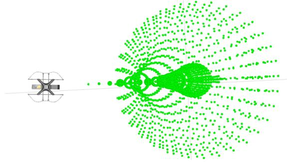
**Figure 10.** A trajectory library (green) of dynamically feasible trajectories as the robot flies to the right at high speed. These trajectories are matched to the local planner A\* path. There are many of these trajectory libraries, which are selected at any time instant according to the current dynamics of the robot in order to maintain the current momentum of the robot.
