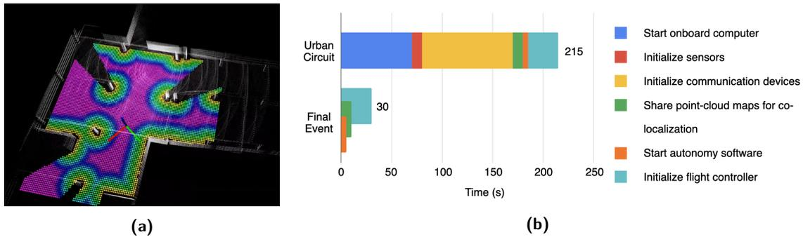
**Figure 17.** (a) A 2D slice of the Euclidean Distance Field for safety check before deploying the drone from the ground robot. The euclidean distance to the nearest obstacles is color coded with purple being the farthest and red being the nearest. (b) Comparison of time profiling for the deployment time in the Urban Circuit and the SubT Final Event.
