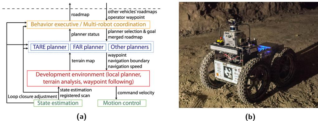
**Figure 11.** (a) System diagram for the ground vehicles used by Team Explorer in DARPA Subterranean Challenge. The system has four layers for multirobot coordination (yellow), task-specific high-level planning (blue), low-level navigation modules (red), and modules for state estimation and motor control (green). (b) One of our ground vehicles (R1) in a tunnel environment.
