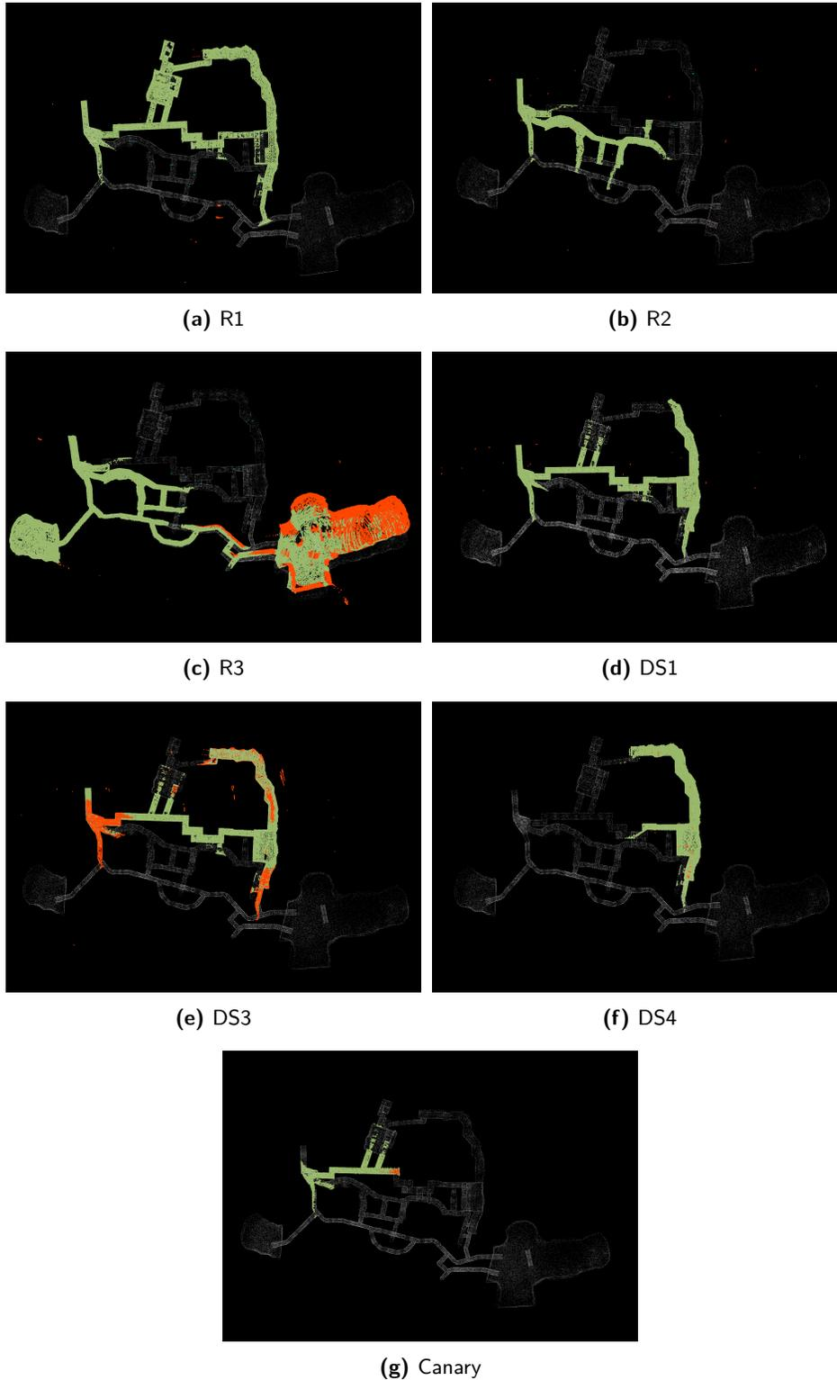
**Figure 27.** Maps obtained by each robot in the Final Round, compared against ground-truth (white) provided by DARPA (Schang et al., ). Green points are registered within a 1 meter mapping tolerance to the ground-truth, while orange points are registered with error greater than the tolerance.
