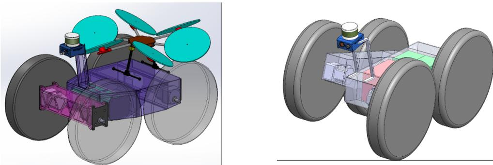
**Figure 3.** Early computer-aided design (CAD) drawings demonstrating the front-to-back and side-to-side suspension approaches. We eventually adopted the front-to-back suspension approach for R2 and R3 because of the bigger chassis allowed for enclosing more electronics and batteries.
