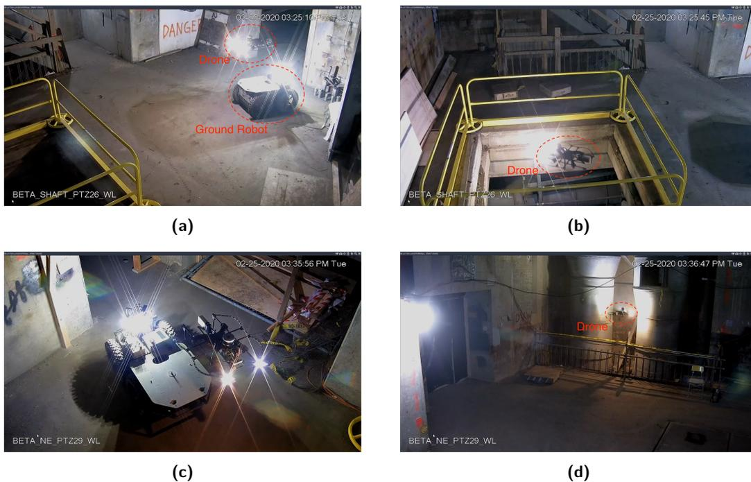
**Figure 16.** (a) The ground robot launched a drone next to a vertical shaft in the SubT Urban Circuit, 2020. (b) After the launch, the drone flew through the vertical shaft to explore the level underneath. (c) Another instance at the SubT Urban Circuit where a drone was launched. (d) After the launch from (c), the drone flew in between and scouted two pipelike structures, the lower part of which was blocked by barriers thus was not accessible by ground robots.
