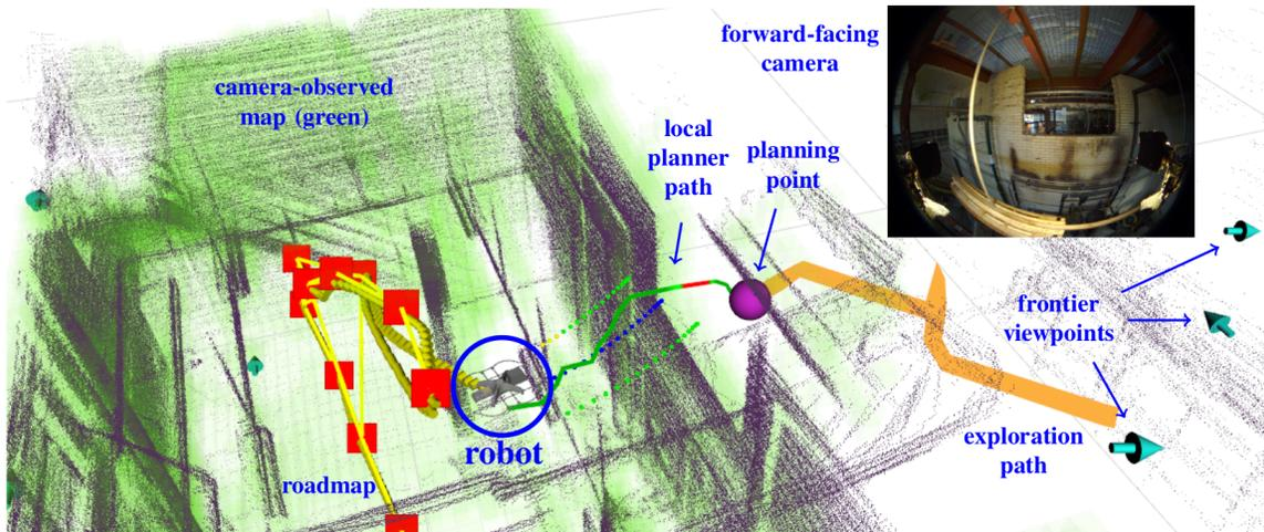
**Figure 7.** Our aerial robot exploring a boiler plant in Pittsburgh, PA. The robot has finished observing the room on the left (green points), so it plans a path between beams hanging from the ceiling and a small hole in the wall (visible in camera field of view) to reach the frontier viewpoints in the unexplored room on the right. All computation is performed online and onboard the robot. The point cloud is generated with our onboard LiDAR sensor and SuperOdometry.
