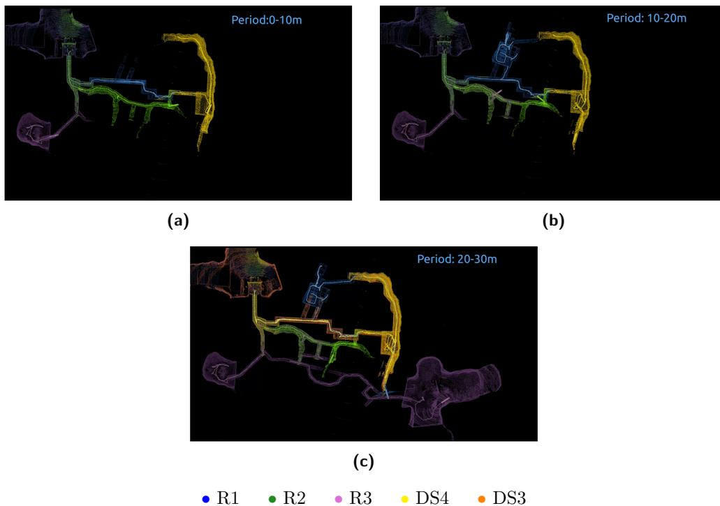
**Figure 24.** Exploration progress in the first 30 minutes. (a) In the first 10 minutes, there were four robots deployed which covered more than half of the environment (about 15 out of 28 sectors). [(b) and (c)] In the first 30 minutes, three ground robots and two aerial robots had already covered more than 80% of the environment (24 out of 28 sectors).
