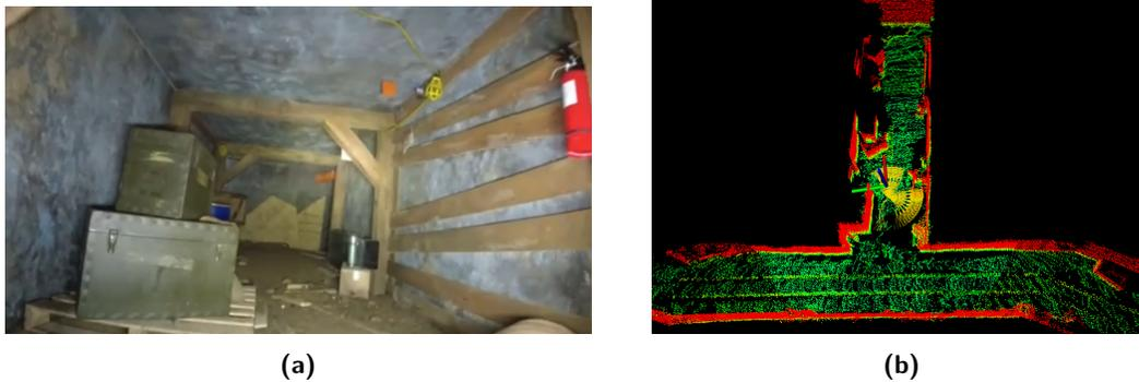
**Figure 12.** (a) Camera view of the environment. (b) The terrain map: green points are traversable areas and red points are nontraversable areas. The coordinate frame indicates the robot's current location. The yellow curves are collision-free paths computed by the local planner.
