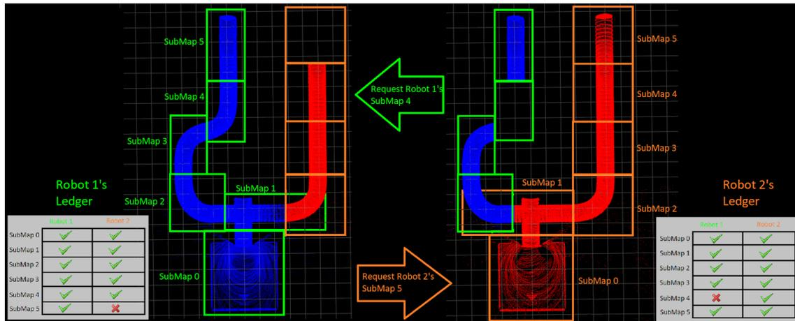
**Figure 22.** An illustrated example of our communication ledger used to store and share information between robots.
