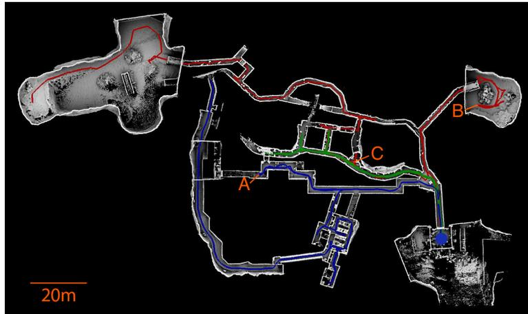
**Figure 14.** Result from SubT Final Event in Louisville Mega Cavern, KY. Three vehicles with red, green, and blue trajectories are deployed running TARE and FAR planners together. The segments between A and B on the red trajectory and between the start point (blue dot) and C on the blue trajectory use FAR planner to transit. Other segments on the trajectories use TARE planner to explore.
