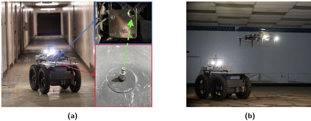
**Figure 15.** (a) The configuration of our wheeled-aerial marsupial system, where a drone is carried at the top of a ground robot. Figures on the right show the latching mechanism used to secure the drone on the launch pad. (b) The instance after the drone is launched. The lights on the drone indicate its heading.
