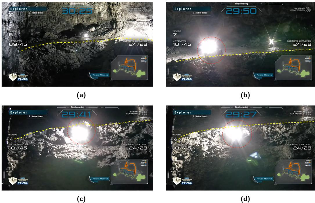
**Figure 32.** R3 fell off a cliff. Dotted circles indicate locations of the robot. The dotted yellow curve indicates the edge of the drop-off. (a) The drop-off, the robot was to the right of the camera view. (b) The robot approached to a rock pile before the drop-off. (c) The robot climbed over the rock pile and detected the drop-off. (d) The robot tried to turn back but slid on loose dirt. It fell down the cliff afterwards.
