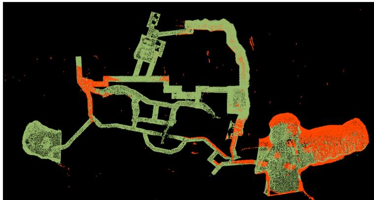
**Figure 29.** Aggregated map deviation of complete map collected by Team Explorer. Green points are within 1 meter tolerance to the ground-truth and orange points are out of the tolerance.
