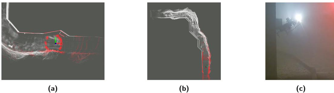
**Figure 30.** DS4 SLAM Issues: It encountered heavy dust in the rail section, which caused SLAM drift and led to collision with the wall. (a) The drone, indicated by the coordinate frame, was surrounded by noise points caused by heavy dust. (b) Misaligned point-cloud map due to the SLAM drift. (c) Camera view of the drone hitting a wall.
