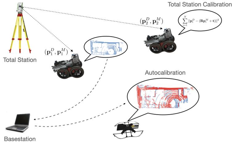
**Figure 5.** Overview of AutoCalibration. At least one robot is calibrated using the total station via least-squares registration, while also sharing a local map to the basestation. Subsequent robots may request this map from the basestation and perform alignment with respect to its own local map
