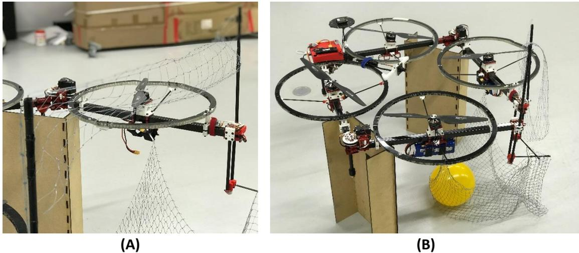
**Figure 4.** (A) Top net made of nylon to block an approaching ball. (B) Bottom net made of polyester to hold the target ball while joints are closed.
