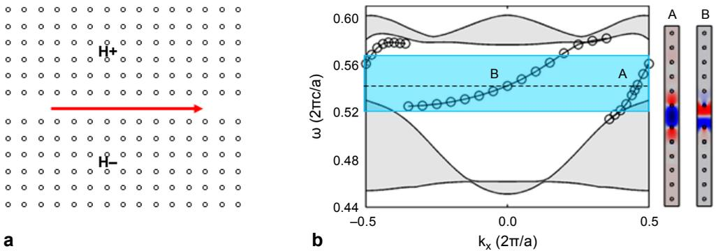
Fig. 1. The UAW structure model (a) and the project bands of the coupled modes (b). The dashed line denotes  $\omega = 0.542$  ( $2\pi c/a$ ) that interacts with the two curves at points *A* and *B*, and the corresponding eigenfields of *A* and *B* are also shown. The project wave vector  $k_x$  is along the waveguide direction.
