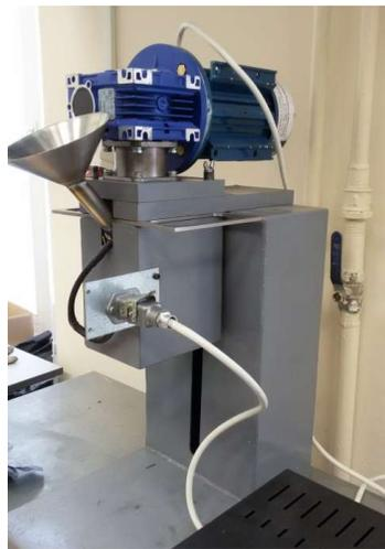
Fig. 2. Laboratory twin-screw mixer
