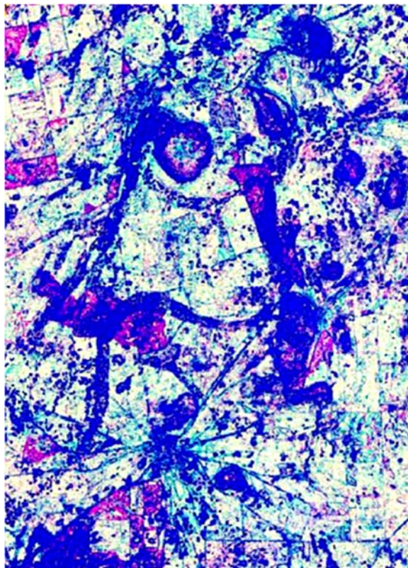
Figure 5. An example of the selection of paleovalleys. The raster is obtained as a result of thematic filtering with subsequent indexing of infrared and thermal channels
