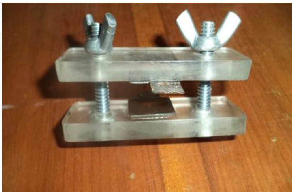
Figure 1. The dry electrochemical cell used for the electrochemical characterization of solid biopolymeric electrolyte films
