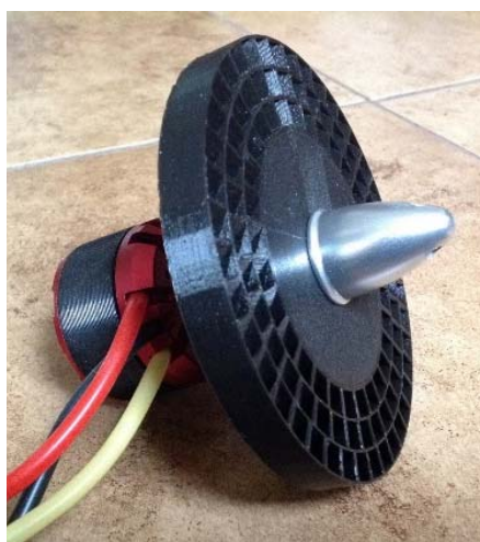
Figure 11. Experimental prototype (pre-production model) of the disk turbine manufactured on a 3D printer for investigating impeller machines with the mesh structure of channels
