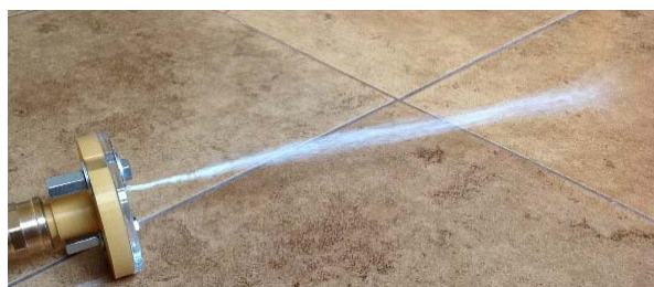
Figure 15. Experimental prototype of the switch-gear equipped with the indicator thread (“ponytail”) when the air flows through the outlet channel for the conditions when the angle \alpha is equal to zero degrees
