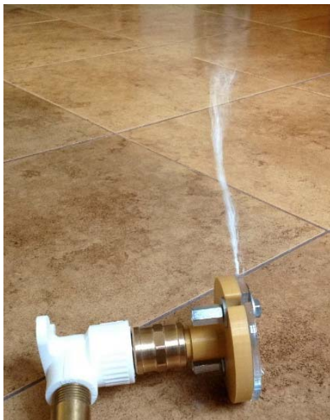
Figure 17. Experimental prototype of the switch-gear equipped with the indicator thread ("ponytail") when air flows through the outlet channel for the conditions when the angle " \alpha " is equal to ninety degrees
