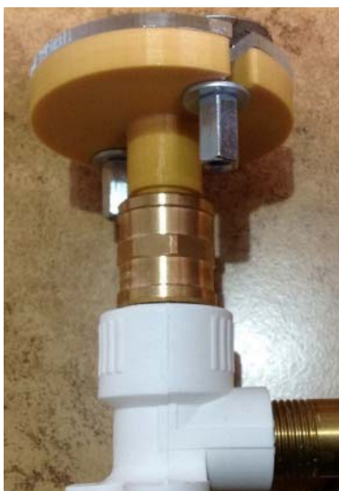
Figure 13. Experimental prototype (pre-production model) of the switch-gear manufactured with the application of additive technologies
