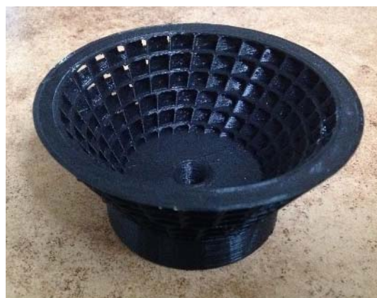
Figure 12. Experimental prototype (pre-production model) of the conical turbine manufactured on a 3D printer for investigating impeller machines with the mesh structure of channels
