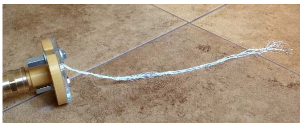
Figure 14. Experimental prototype of the switch-gear with the indicator thread (“ponytail”) when the air current is cut off
