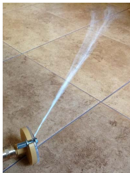
Figure 16. Experimental prototype of the switch-gear equipped with the indicator thread (“ponytail”) when air flows through the outlet channel for the conditions when the angle \alpha is more than zero degrees but less than ninety degrees
