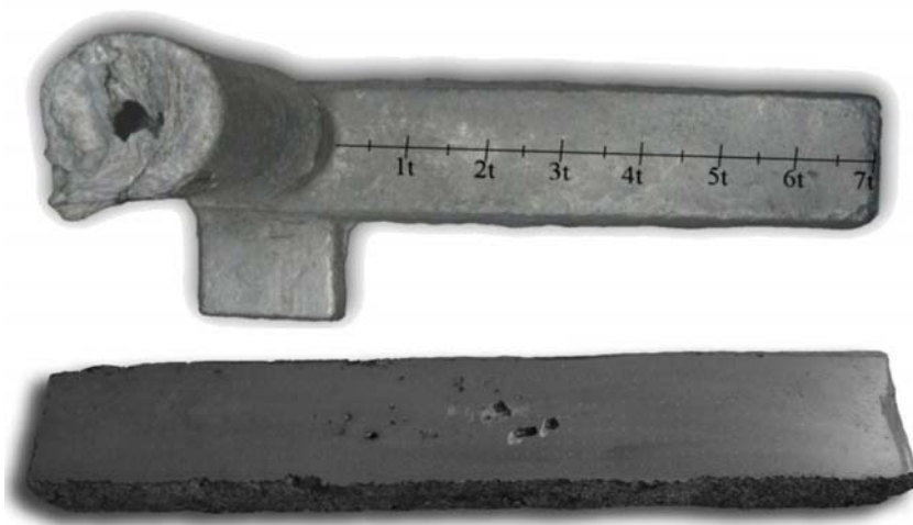
Figure 2. Flow test and preparation for the testing template
