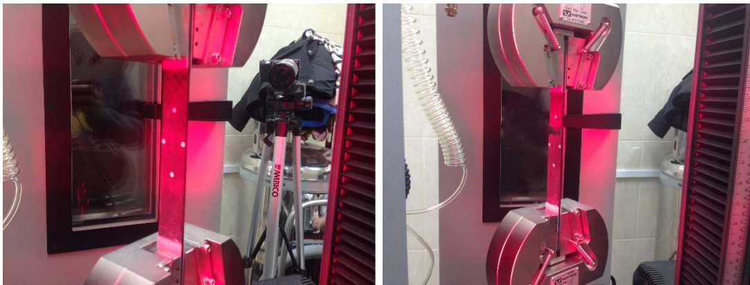
Figure 4. Labeled tensile test sample mounted in mechanical grips before and after the test
