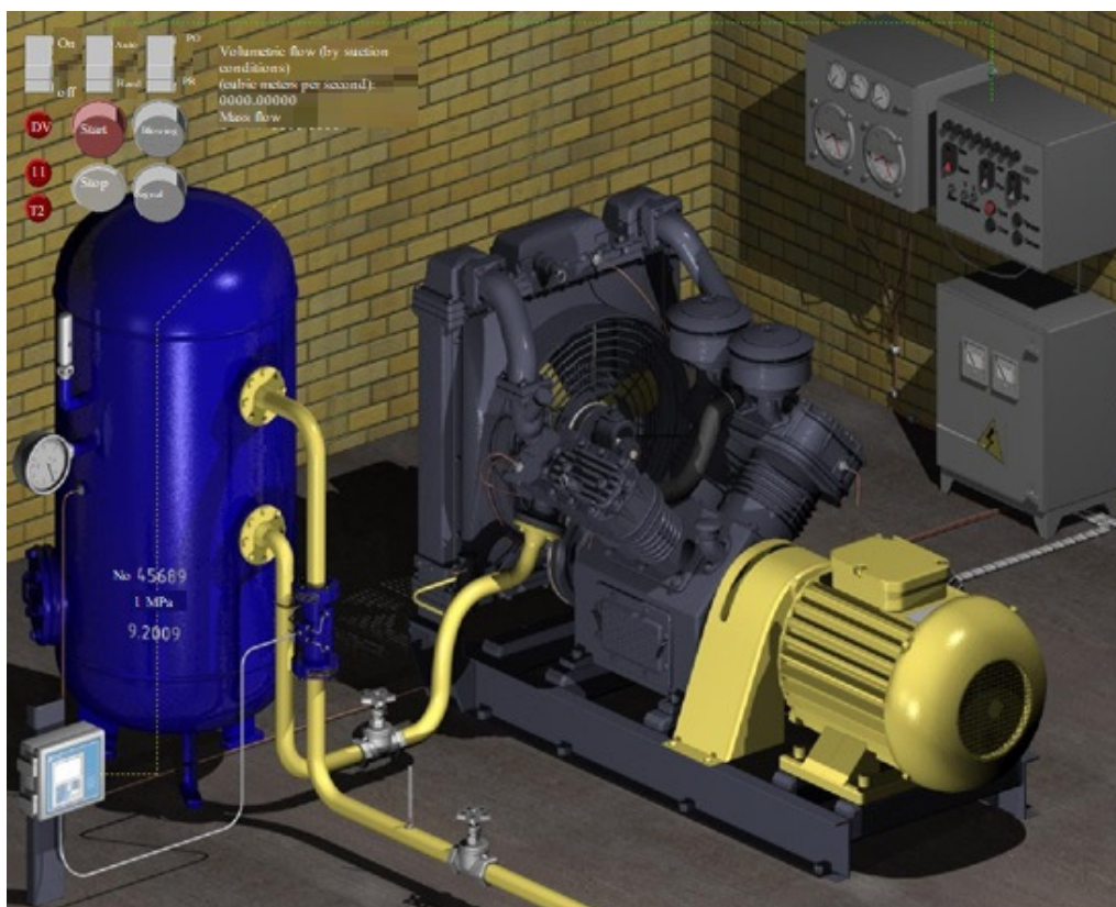
Figure 4. Virtual laboratory work on starting the compressor
