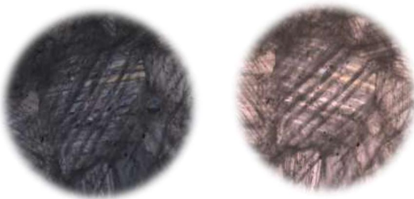
**Fig 1:** Zoom in of 10x10,  $\varnothing=2\text{mm}$ , displaying a massive texture, granoblastic structure, and identified as calcite marble.
