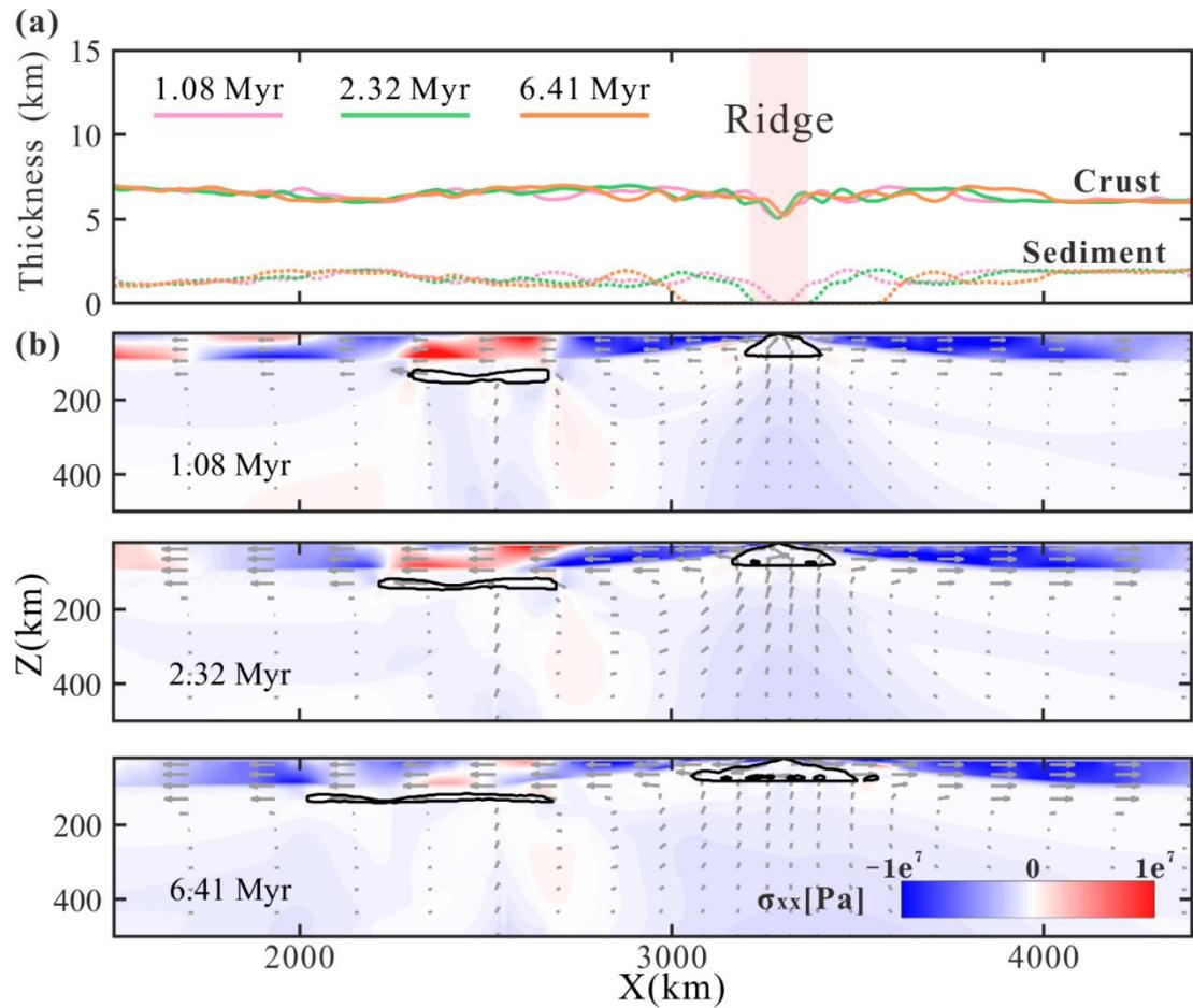
**Figure S4.** Reference model (M77, see Table S1, same as Fig. 4) evolution of plate-drag plume flow shown by (a) crust and sediment thickness, (b) normal stress. The mantle plume weakens the overlying oceanic plate and changes the stress state of the overlying oceanic plate. Molten plume material beneath the lithosphere is extracted to the crust.
