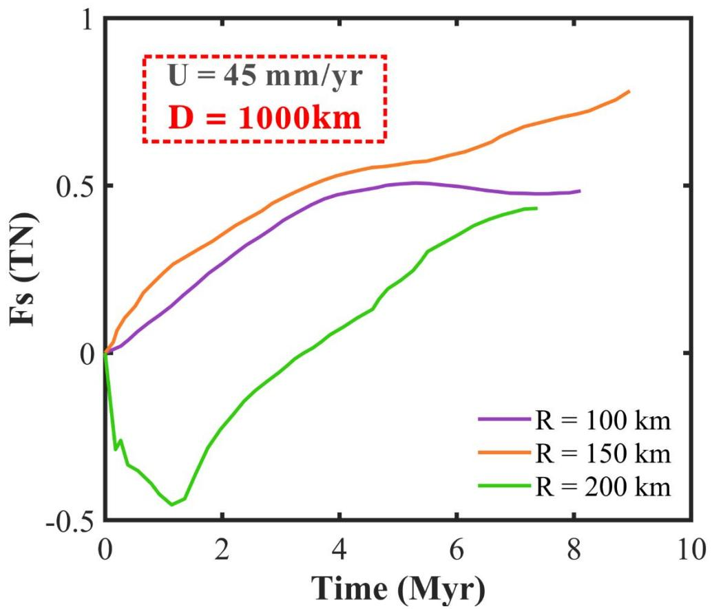
**Figure S7.** Shear force ( $F_s$ ) between plate and plume in different plume head size models. The shear force imposed on the plume increases with plume size. The negative shear force indicates stronger friction imposed on the ridge-ward flowing (right) plume branch than that on the plate-drag flowing (left) plume branch.
