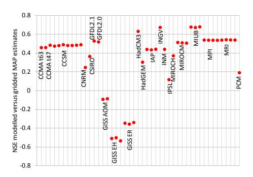
Fig. 2. Nash–Sutcliffe efficiency (NSE) values for modelled vs. observed MAP untransformed estimates.
