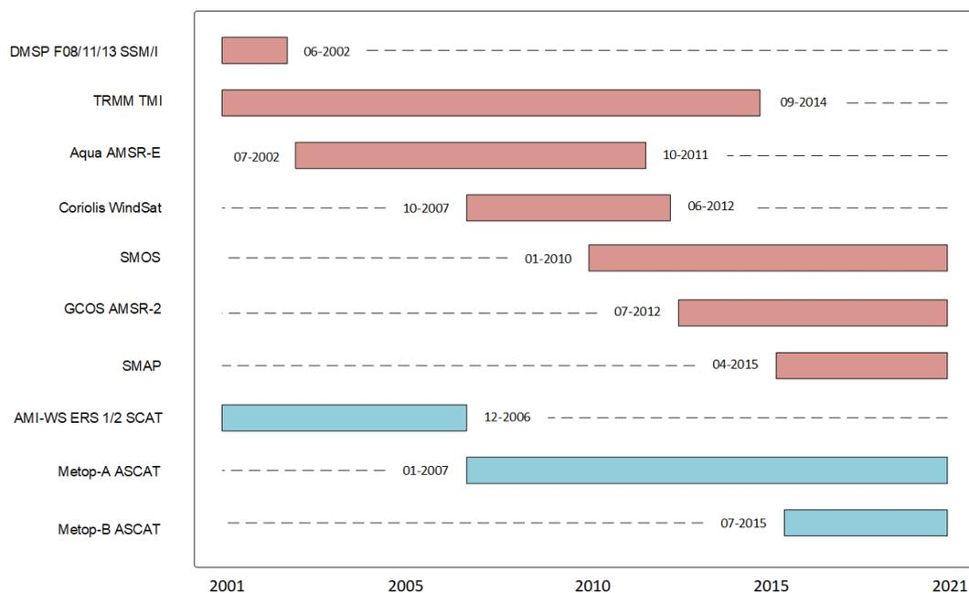
**Figure 1.** A timeline of satellite missions utilized in the C3S v202012 dataset during the period 2001–2020. Passive sensors (radiometers) are represented by red bars, while active sensors (scatterometers) are represented by blue.
