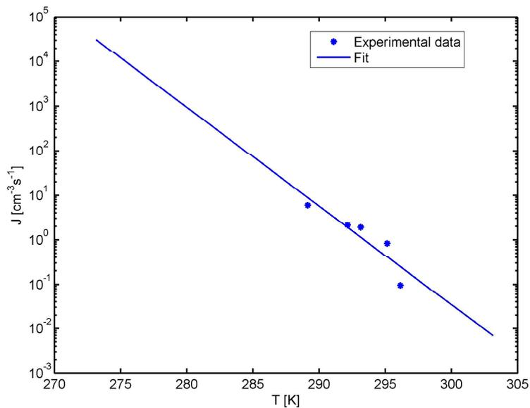
**Fig. 1.** Particle formation rates calculated from the particle number data for different temperatures in the flow tube (IfT-LFT) at r.h.=28% (asterisks) and the fitted line, which was used to extrapolate the temperature dependence to  $T=273$  K.
