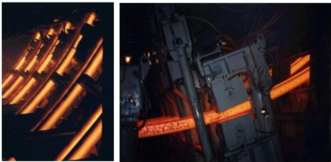
Figure 3: Strand unbending by straightener withdrawal units during secondary cooling zone of continuous casting process of steel [37]
