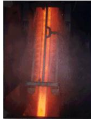
Figure 4: Secondary cooling stage in continuous casting steel
