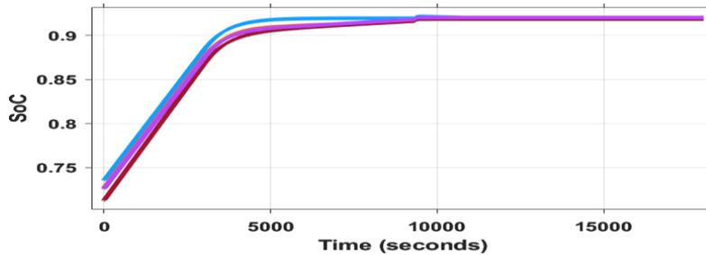
Fig. 19 SoC balancing during charging phase.
