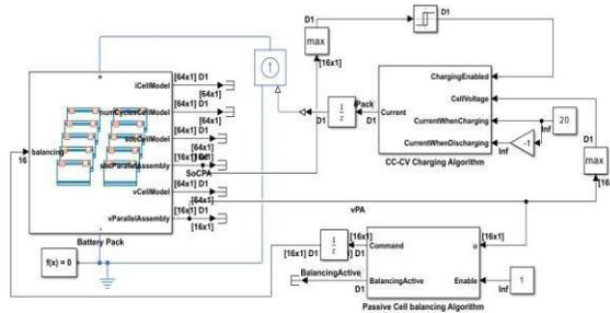
Fig.16 System Modelling of battery pack with passive cell balancing and charging/discharging.
