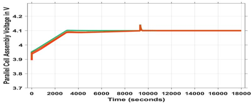
Fig. 20 Parallel assembly voltage during charging
