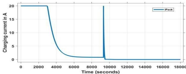
Fig.21 CC-CV charging waveform
