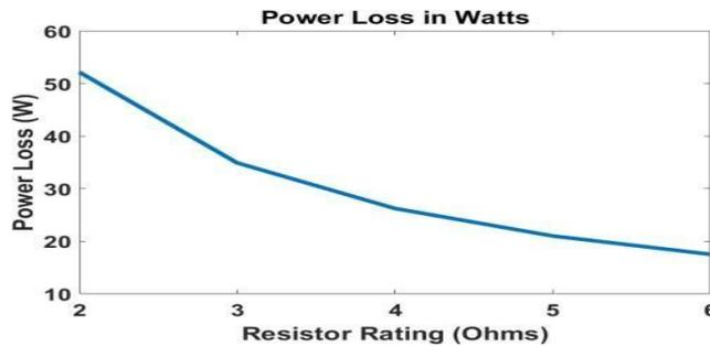
Fig.13 Power loss variation with shunt resistor.
