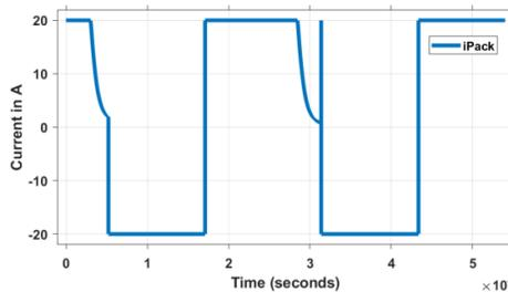
Fig.17 battery pack current during charging and discharging.
