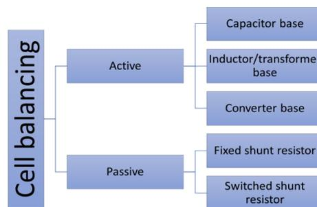
Fig.2 cell balancing classification.
