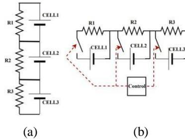
Fig. 3 Shunt resistor a) fixed resistor b) Switched shunt resistor.
