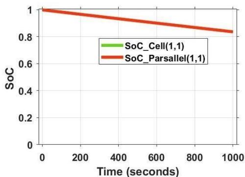
Fig. 8 State of Charge (SoC) Variation during discharging phase of the battery cell.
