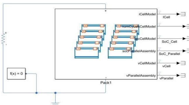
Fig. 7 Battery pack connected to a load resistor for discharging.
