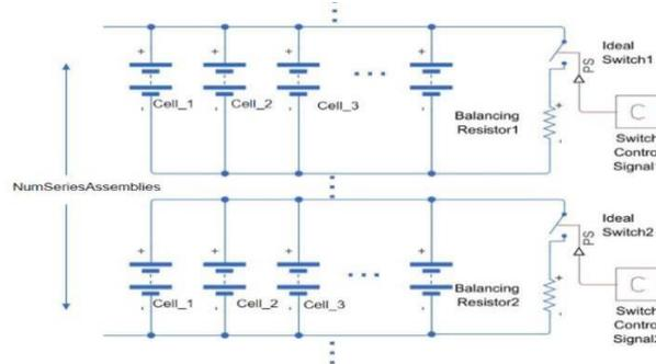
Fig. 10 Passive cell Balancing circuit.
