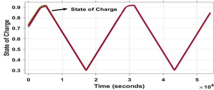
Fig. 18 Variation of SoC with time during charging and discharging
