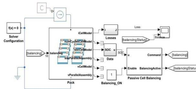
Fig. 11: System level modelling of battery pack with Passive cell balancing circuit.
