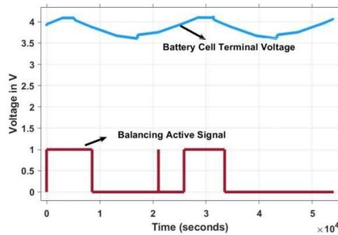
Fig.17 Battery Cell terminal voltage during charging and discharging
