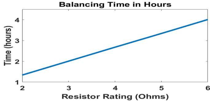
Fig.12 Balancing time variation with shunt resistor.
