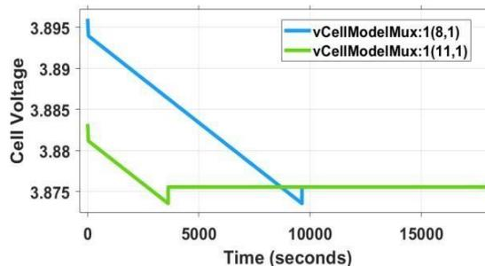
Fig. 15 The variation of terminal voltage of battery pack for a balancing resistor of 4 ohm.
