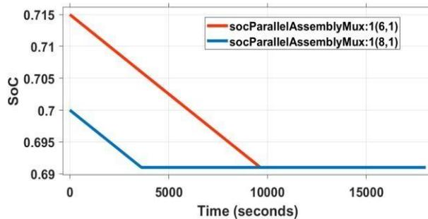
Fig. 14. The variation of SoC of battery for a balancing resistor of 4 ohm.
