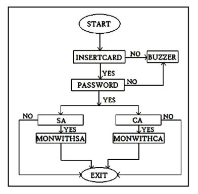
Fig.1 Flowchart of VHDL code of specified ATM functioning
