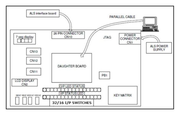
Fig.3 Connection diagram of Base-Board
