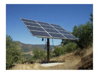
Figure 1. Two Axis Solar Tracker
