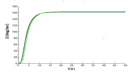
Figure 9. Real and observed Angular velocity of the altitude motor
