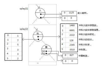
Figure 4. Sample of splay trees in stable state
