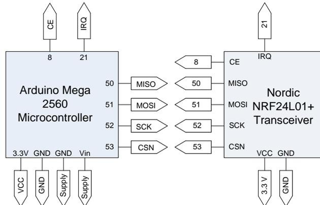
Figure 1. Hardware wiring of the sensor node.
