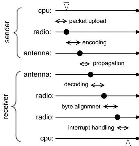
Figure 3. The timing of the transmission between the sender and the receiver.
