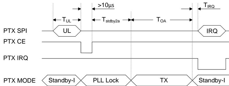
Figure 4. Timing sequence of the nRF24L01+ radio module[20].
