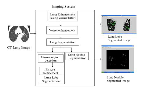
Figure 3.Block Diagram
