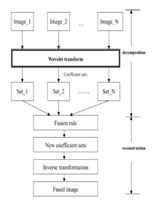
Figure 2: The flowchart of wavelet image fusion
