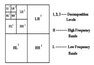
Figure 3: Structure of 2-D DWT with 3 decomposition levels
