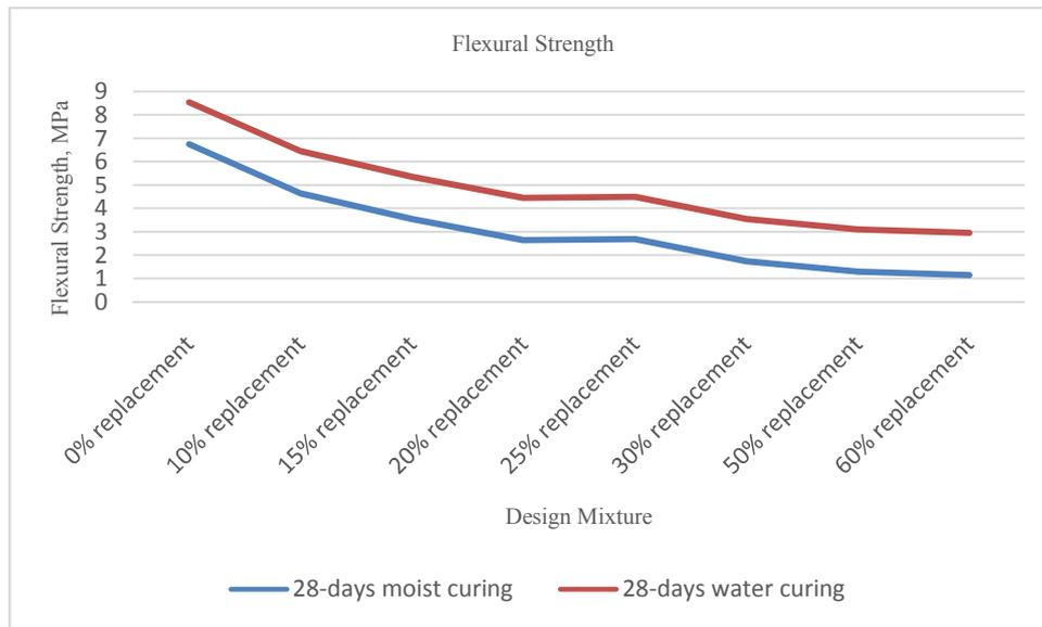
**Figure 2. Comparison of Flexural Strength on Curing Method**
