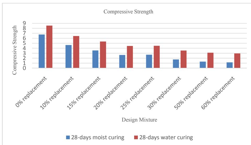
Figure 1. Comparison of Compressive Strength on Curing Method
