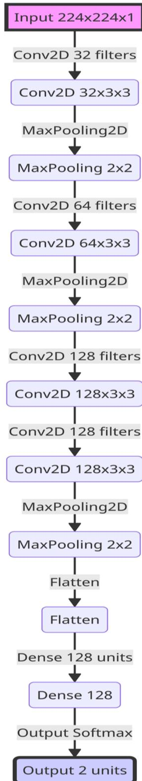
**Figure 1:** Flow diagram of CNN-based binary classification
