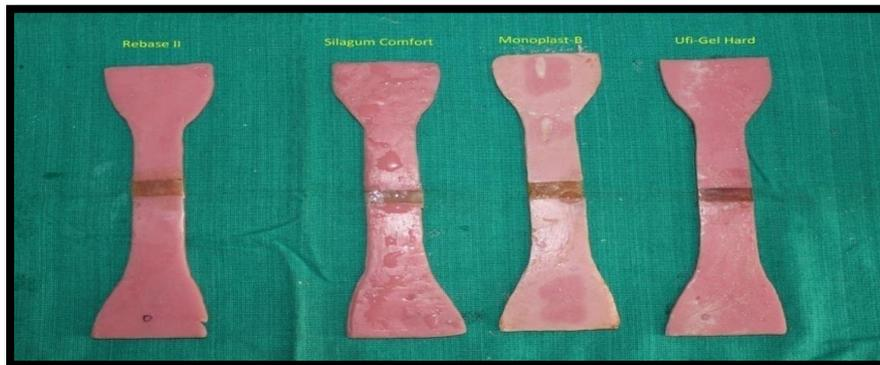
**Figure 8:** Test Specimens from each group
