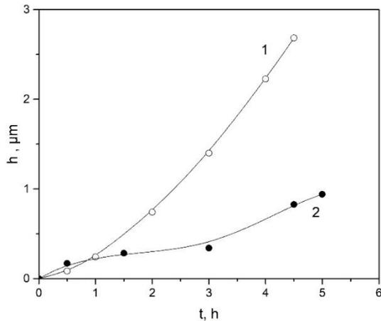
Fig. 5. Kinetic wear curves for the samples VT6 ( $h_c$ ) from the cavitation time before and after ion-plasma modification ( $t_p$ ): 1 –  $t_p = 0$ ; 2 – 15 min
