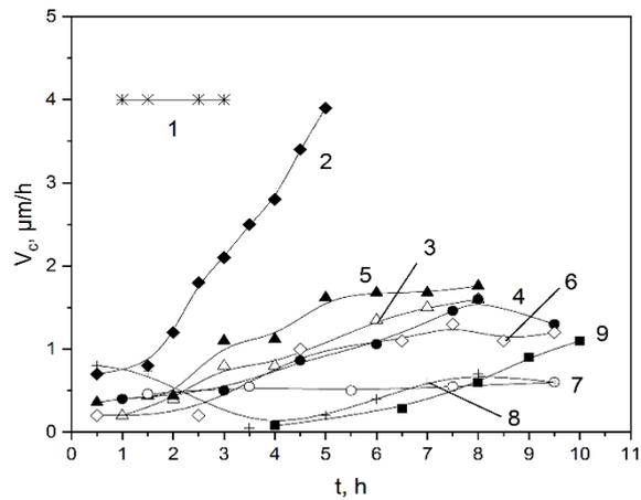
Fig. 4. Average wear rates of samples from different titanium alloys (see Table 2) depending on the cavitation time
