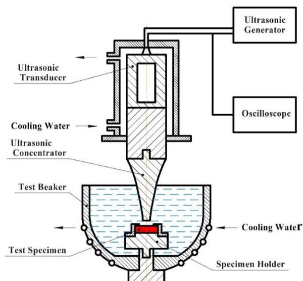
Fig. 1. Schematic diagram of the experimental stand for cavitation
