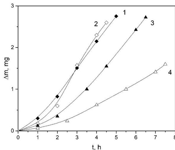
Fig. 2. Dependence of wear ( $\Delta m$ ) for the samples VT1-0 on the cavitation time ( $t$ ):
