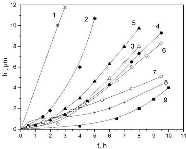
Fig. 3. Dependence of the average depth of erosion for titanium alloys on the cavitation time: 1 – VT1-0; 2 – TC5; 3 – VT6; 4 – VT14; 5 – OT4; 6–9 – after modification of VT6 and VT14 samples (Table 2)
