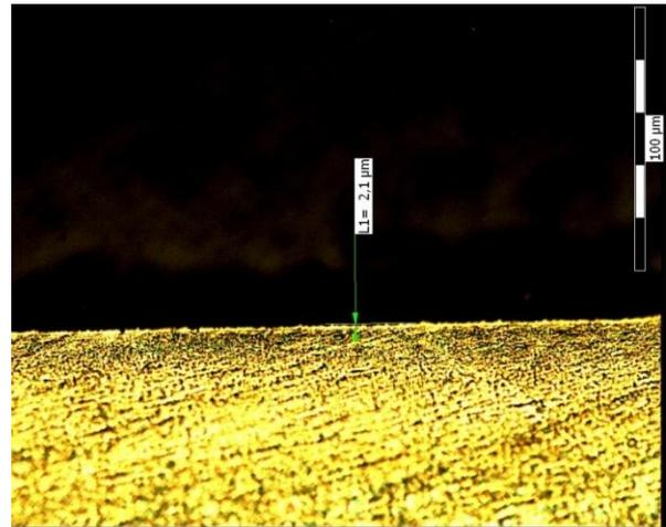
Fig. 7. Optical microscopy of the VT-6 alloy cross section after 15-minute ion-plasma modification
