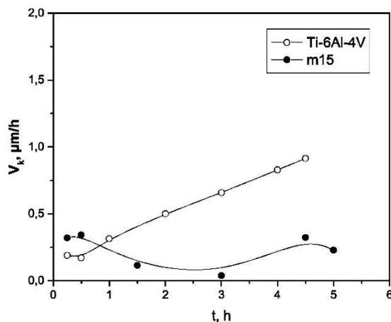
Fig. 6. The dependence of the cavitation wear rate for VT6 alloy on the cavitation time for the initial samples and the samples modified with plasma ions for 15 min
