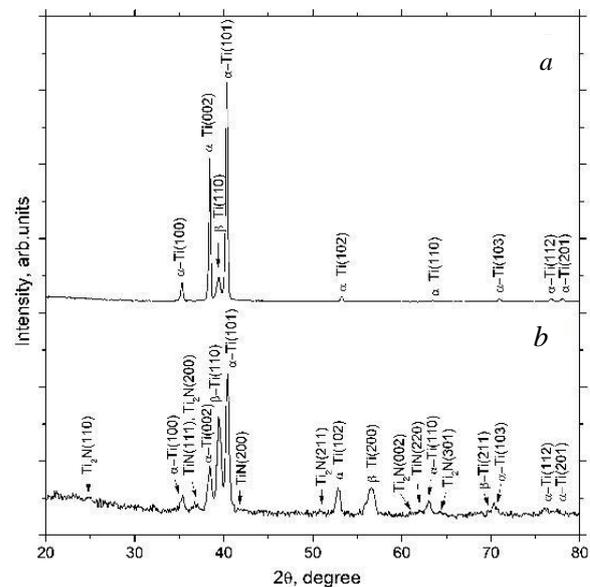
Fig. 8. Diffractograms of the VT6 sample: a – initial; b – after 15-minute ion-plasma modification
