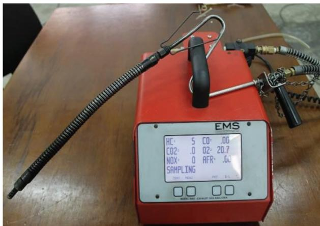
Figure 4: Emission gas analyser (EMS)
