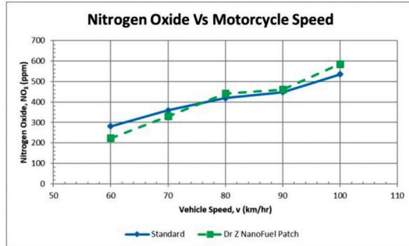
Figure 8: Graph of nitrogen oxide against motorcycle speed
