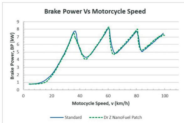
Figure 6: Graph of brake power against motorcycle speed
