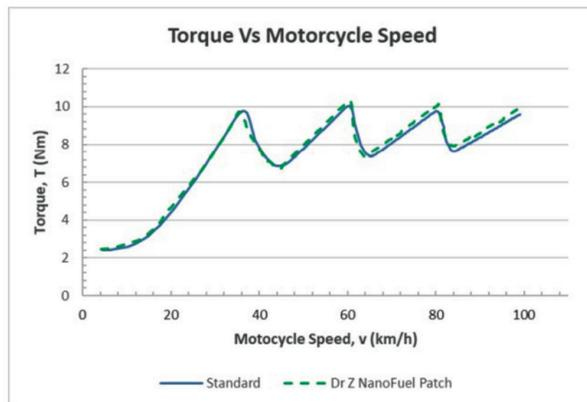
Figure 5: Graph of torque against motorcycle speed
