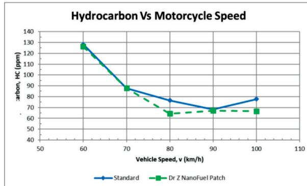
Figure 10: Graph of Hydrocarbon against engine speed
