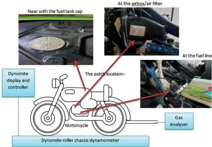
Figure 2: Schematic experimental setup of Dynomite roller chassis dynamometer. The test was repeated at least three times to obtain reliable data
