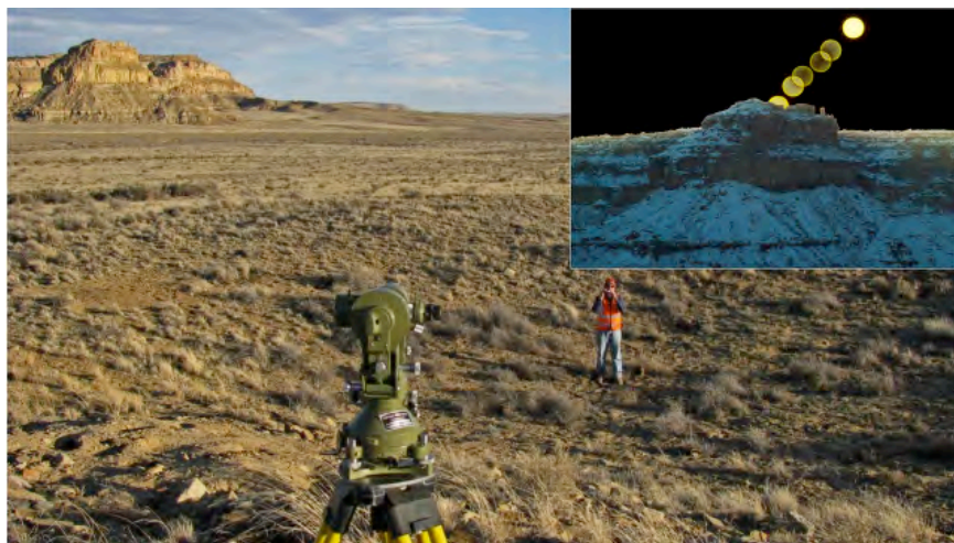
Fig. 1. Theodolite at the edge of the Great Kiva of Marcia's Rincon. The theodolite is located at the back sight above the likely antechamber of the unexcavated structure. Inset: Filtered images of December Solstice Sunrise over Fajada Butte. Both photographs by Ninnemann.
