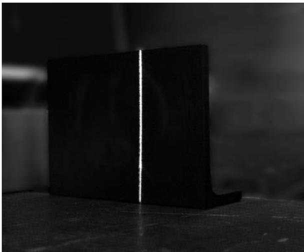
Fig. 5 Light line images on the reference plane during calibration
