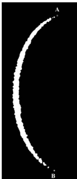
Fig. 5 Image of cylinder in light of laser section
