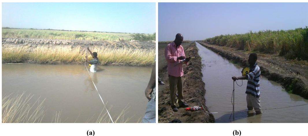
Figure 2: Cross section and velocity measurement of typical monitored primary canal 2 (a) and tertiary canal 611 (b).
