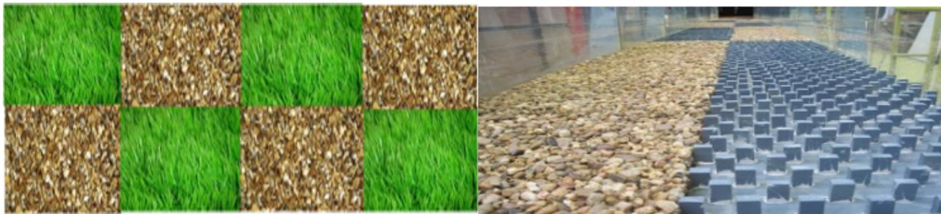
Figure 2: Bed roughness configuration plan view of roughness patches for experiment one and two.
