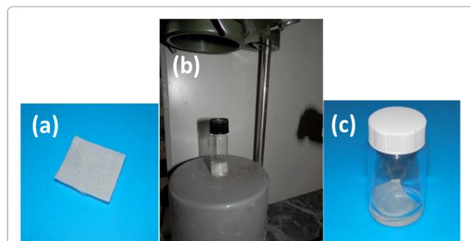
**Figure 1:** Fabric phase sorptive extraction: (a) a fabric phase sorptive extraction (FPSE) device; (b) extraction using FPSE device; (c) solvent mediated back-extraction.
