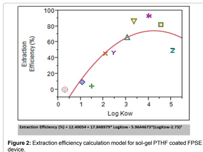
**Figure 2:** Extraction efficiency calculation model for sol-gel PTHF coated FPSE device.
