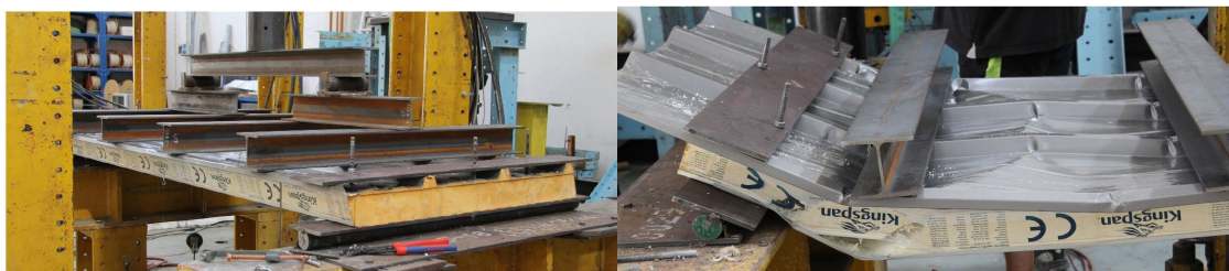
Figure 4. Specimen, left: before test, right: after test (failure of panel core)
