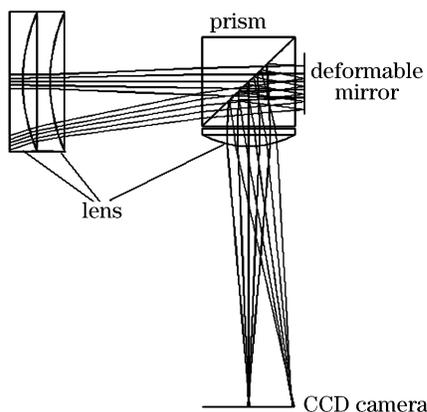
Fig. 1. Final optical system design.
