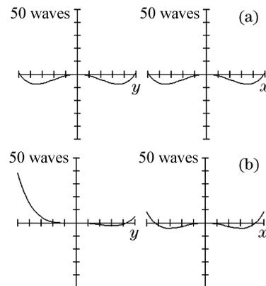
Fig. 2. Wavefront error (OPD versus normalized pupil) without correction at the FOVs of (a)  $0^\circ$  and (b)  $30^\circ$ .
