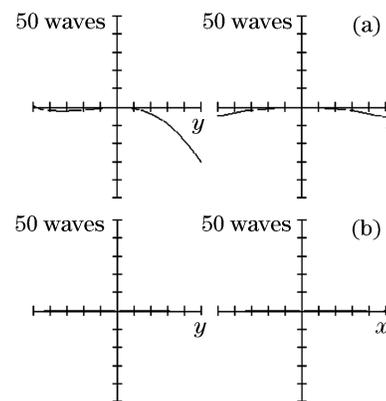
Fig. 3. Wavefront error with correction at the FOVs of (a)  $0^\circ$  and (b)  $30^\circ$ .
