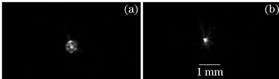
Fig. 6. (a) Uncorrected and (b) corrected images of a 20- $\mu\text{m}$  pinhole at a 25° field angle.
