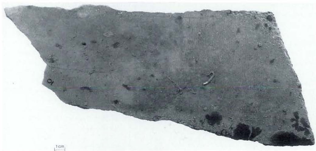
Fig. 2. Block no. 8, a thin slab polished on both sides and rough around the edges. This was on the seafloor at -8 m at locality 11 for 2 years. \times 0.5 .
