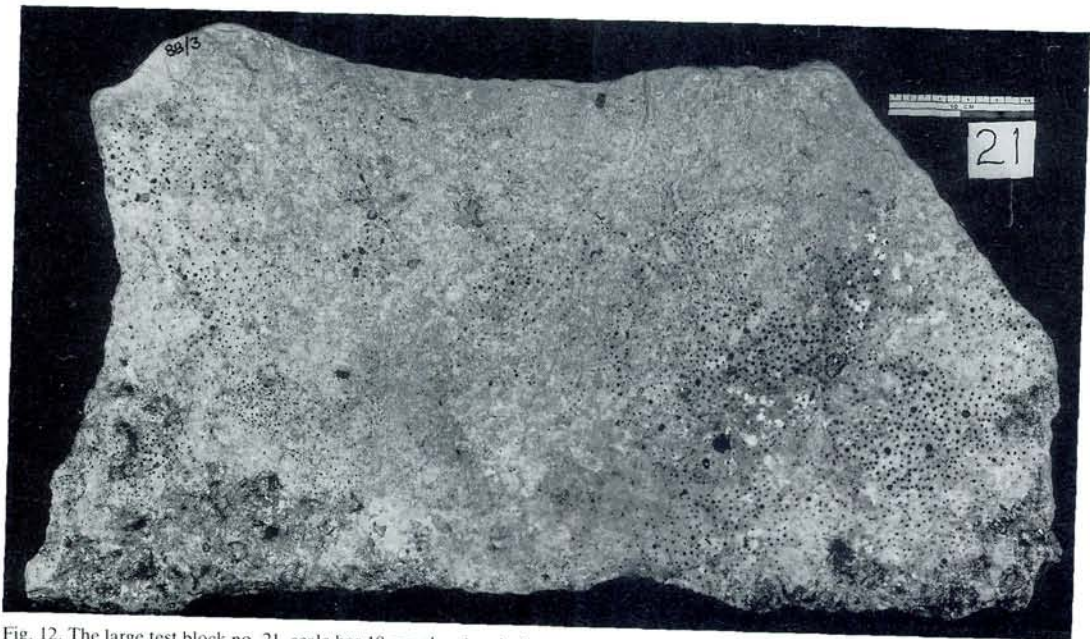
Fig. 12. The large test block no. 21, scale bar 10 cm, showing the lower surface. All parts are irregular fracture surfaces. The block lay on the seafloor at locality 14 in \sim 3 m for 5 years and has been extensively colonized by boring sponges.
