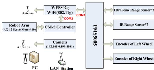
Fig.3. System Hardware Interface.
