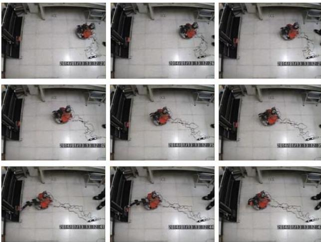
Fig.10. Moving and Scanning to find Target and Grab Target.
