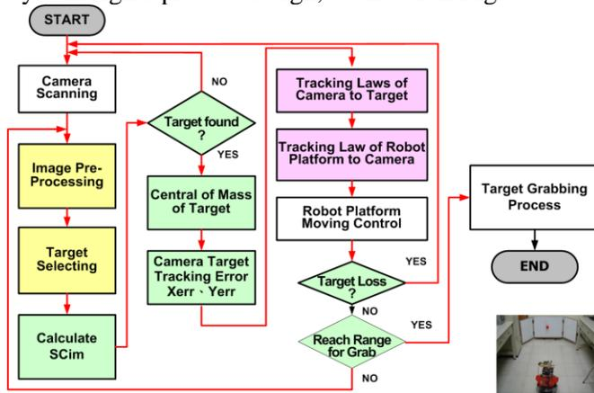
Fig.7. System Operation Flow Chart.
