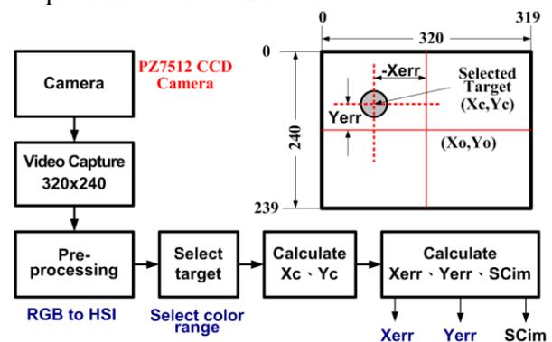
Fig.8. Data Processing Flow Chart & Parameter Definition.
