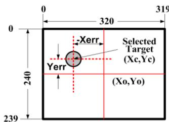
Fig.6. Tracking error definition of the Target.
