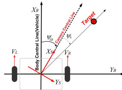
Fig.4. Relationships between Target, Camera and Platform (Vehicle).
