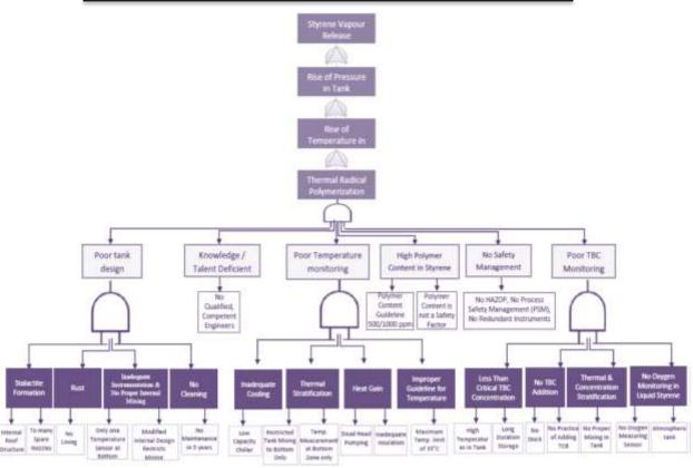
Fig 5: Fault Tree Diagram (FTD) explaining Styrene Vapor release
